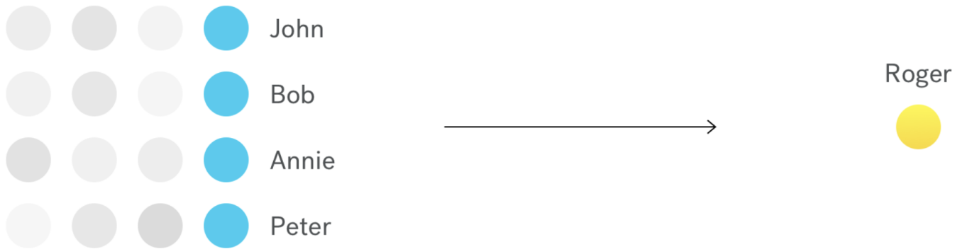
Figure 2.1: The identity of the signer is obscured. For example, if you encounter a ring signature with the public keys of Annie, Bob, John, and Peter, you will be able to claim that one of these users is the signer, but not be able to pinpoint him or her.
